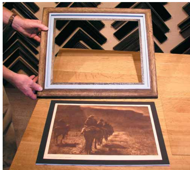
To buffer the print from the glass, a hidden or "gasket" mat was used, with the bevel reversed. The rabbet is cut wide to accommodate a slightly narrower mat and is sealed with frame sealing tape.
