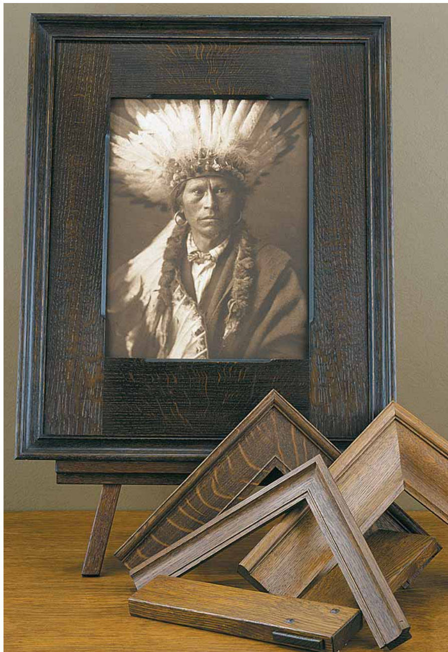
This original photogravure of Edward Curtis's "Chief Garfield" was close-framed, with 3" margins all around the image hidden. This oak frame used stop chamfers to soften the sight edge. Samples of other quarter-sawn oak frames used for close framing are also shown.
