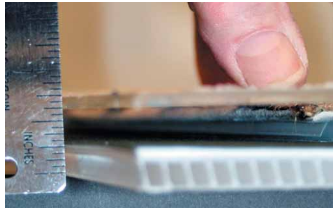
Measure the thickness of the assembled mounting package to determine the depth of spacers between the acrylic overlay and the solid backing board, in this case \frac{3}{4} ". Hand-applied pressure compresses the polyester batting and provides slight tension between the sampler and the acrylic overlay. After removing masking from the acrylic and installing a spacer on the acrylic sheet's edges, final fitting is all that remains to be done.
