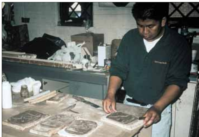
Photo 2: The compo cross straps are sliced and applied while warm and pliable. The antique book press is still the best way to make the cross straps, as Gold Leaf Studios artisan, Koy Eam, slices the compo with a thin gilder’s knife. (photo credit: William Adair)
