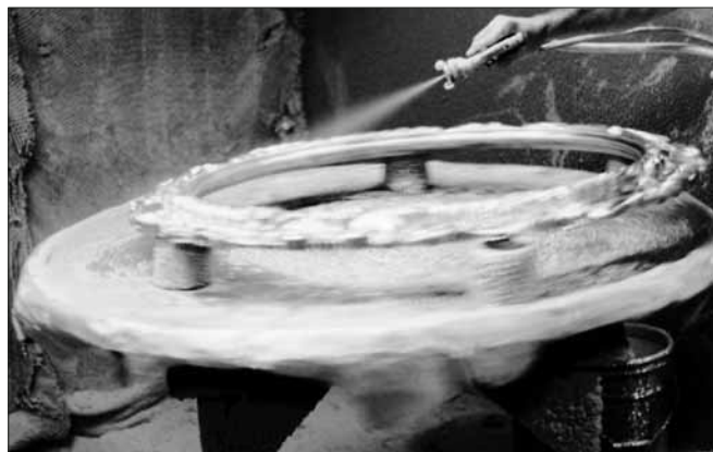
Photo 13: A silvered frame is sprayed with gold tint dye as it spins.
