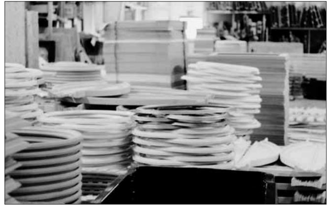
Photo 10: These stacked frames have been sprayed with undercoat and are waiting for finishing.
