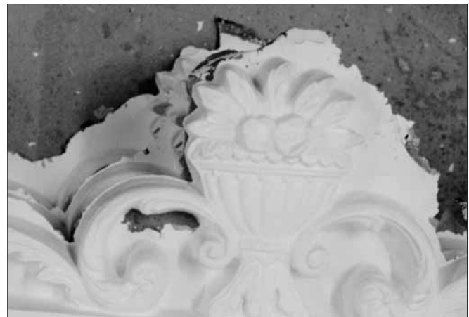
Photo 8: This is a cast frame waiting for the sander. The flashing around the edges is removed in the sander.
