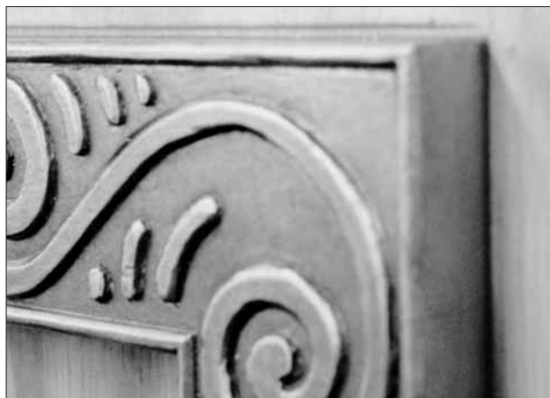
Photo 1: The frame pattern is attached to plywood.
