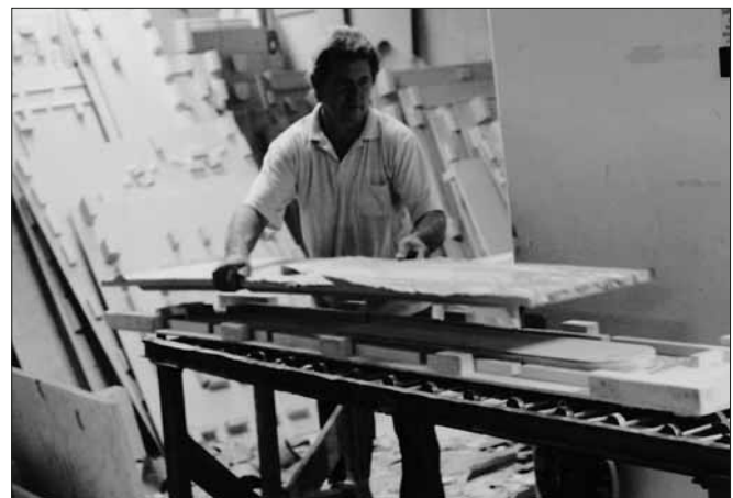
Photo 9: A door panel is being placed in cradle before sanding. Other cradles are in the background, with frames.
