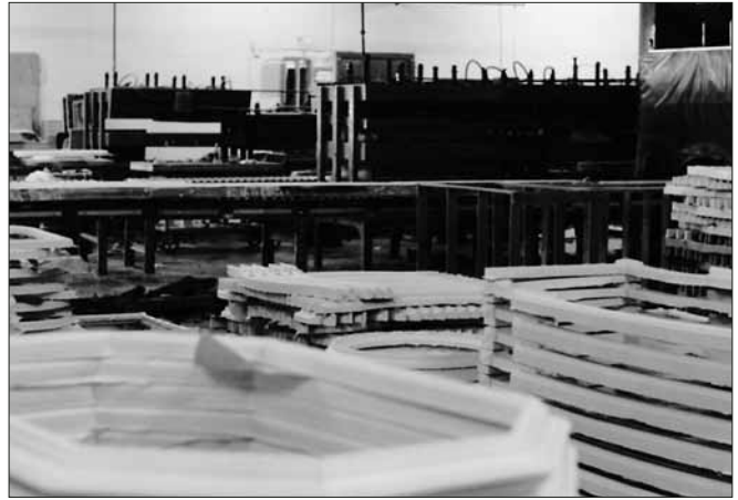
Photo 7: Cast frames are stacked near press used to cure frames.
