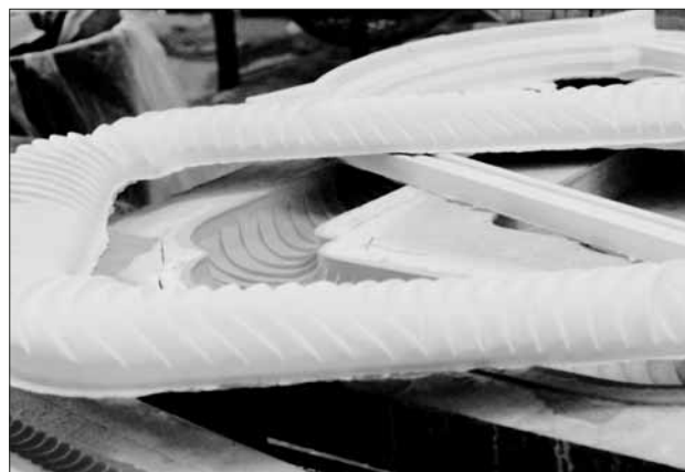
Photo 3: Polyurethane castings are resting on top of silicone rubber molds and slip boxes.
