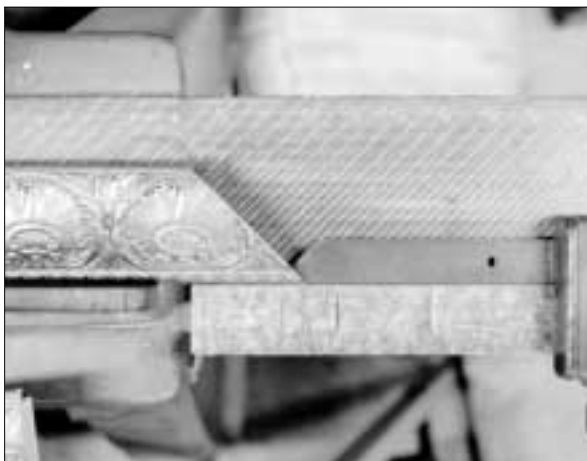
Photo 8: The farthest point on the measuring stop is where the moulding sets on the stop.
