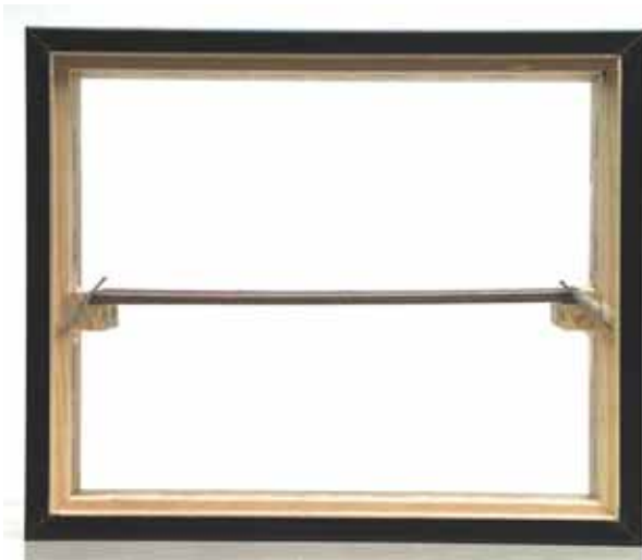
Diagram E: Staple the masonite into the moulding edge and toenail the shelf in the frame. We recommend two staples on each side to ensure no shelf movement.
