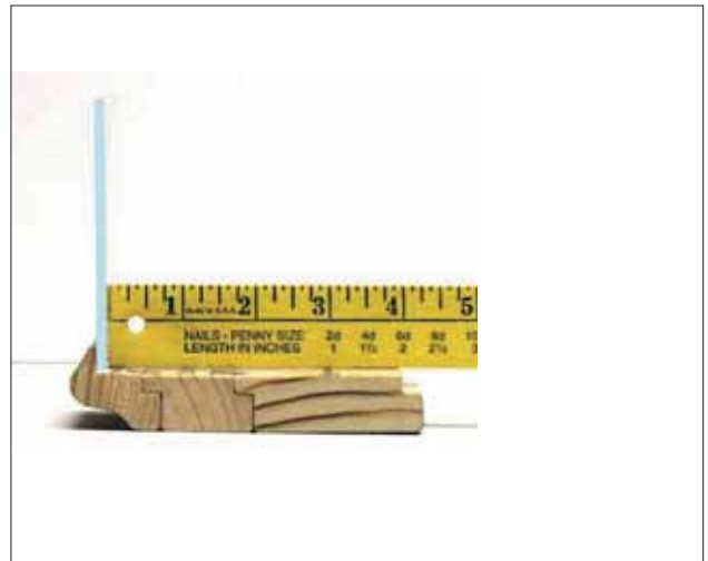
Diagram B: To determine the depth of the shelf, measure from the glass to the backing board. You won't want the shelf to touch the glass, so deduct \frac{1}{4} " to \frac{1}{2} " from your measurement.
