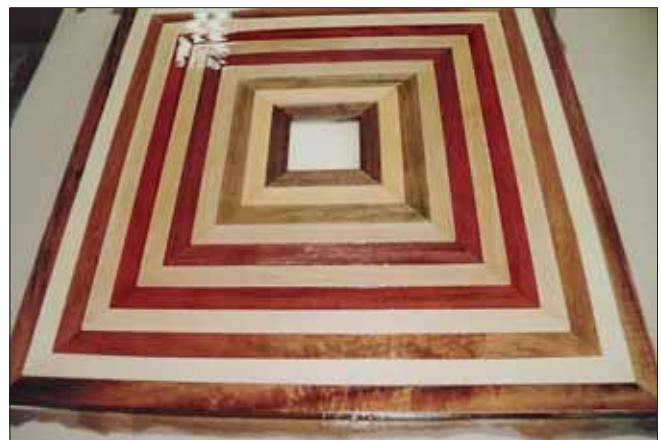
Oil has been applied. Let it sink and soak in the wood.
