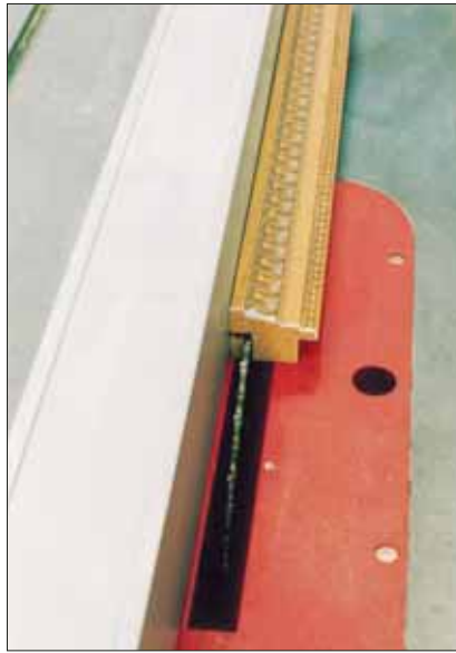
Photo 5: Here, a table saw is being used to cut out a second rabbet as described in method one.
