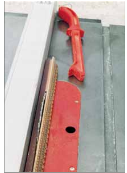
Photo 6: A table saw can also be used to remove all of the wood below the face of the moulding, as described in method two..
