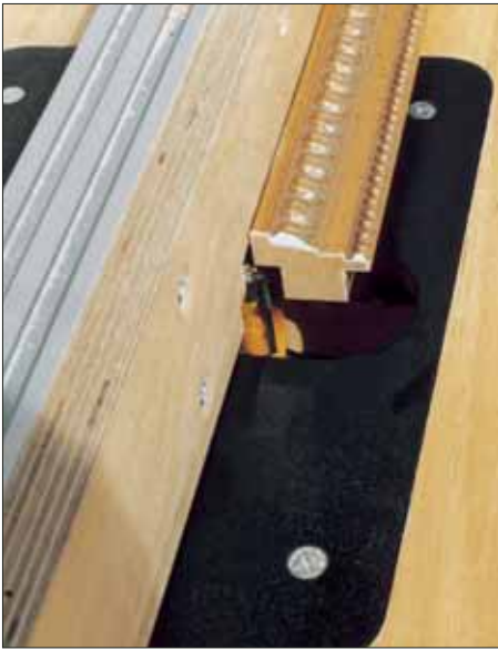
Photo 4: Here, a second rabbet is being routed to be the same height as the existing rabbet, as described in method one..
