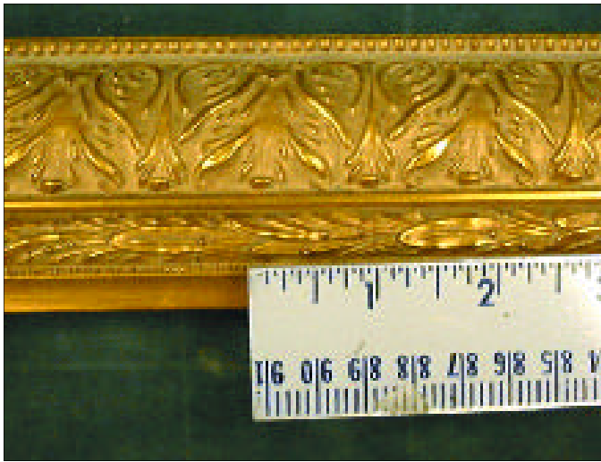
Photo 1: Multiply the total cuts by the inches between the repeat in the moulding pattern.
