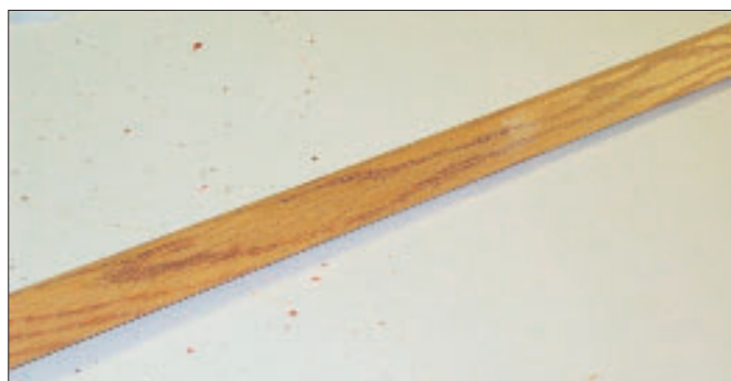
Photo 4: Red patinating wax, applied on the left portion of the moulding, emphasizes the grain pattern of the wood.
