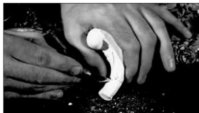
Step 7: Scoring the ornament with an X-acto knife so that it will snap easily.
