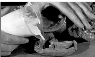
Step 4: Pouring Hydrocal into the newly made mold.
