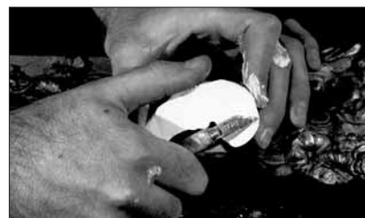
Step 9: Shaving the back of the ornament so that it will be level.
