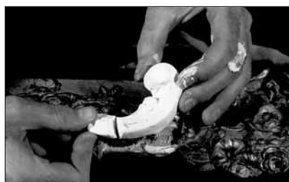
Step 8: Breaking the casting along the score line.
