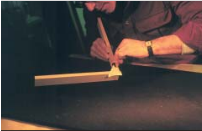
Glue the square of silk to your frame, then trim the excess.
