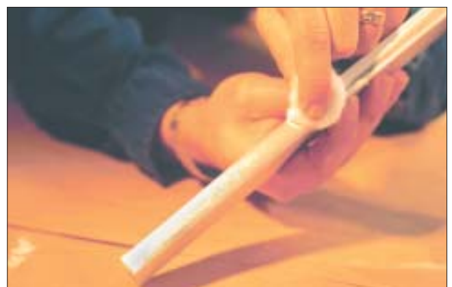
Wipe off the whiting and lacquer thinner paste with a cotton ball.
