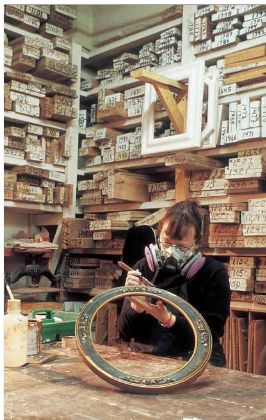
Kristin Nelson-Baird works on restoring a frame in the shop area. Behind her are a portion of the company’s molds used to make compo corners and other ornaments.
