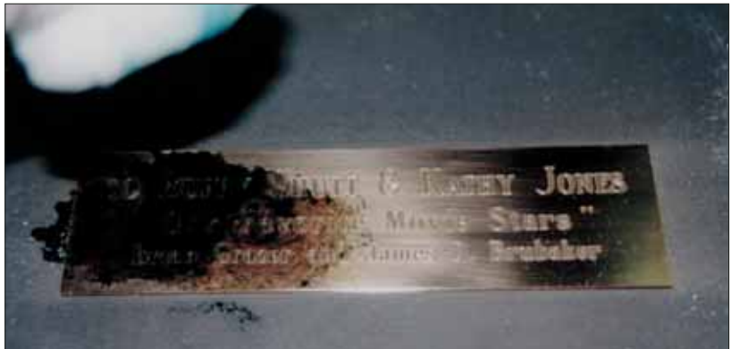
Photo 6: Apply the oxidizing agent and let sit for five to 30 seconds.
