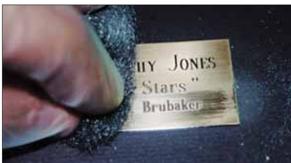
Photo 3: Remove the protective varnish with a steel wool pad.
