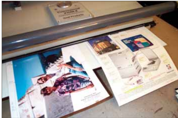
Photo 2: Test Strips—Images were divided into sections that were subjected to timed heat exposures, so comparisons could be made within the context of all temperatures on one tested image.
