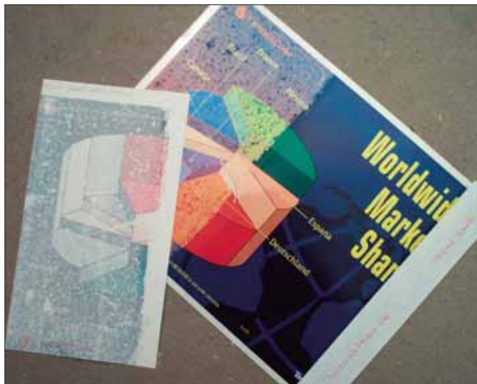
Photo 3: Melted Image—The left hand piece is a segment of the single-sided release paper used in the heat test of this Tektronix 240 thermal transfer image onto film. Notice the inks have melted and transferred to the release paper (left) under the 170°F temperature also severely damaging the original (right).
