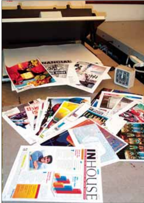
Photo 1: Test Samples—All digitals were mounted in a Seal 210M-X mechanical press for one minute at temperatures ranging from 150°F to 220°F. Samples represented include all common digital technologies that might be suitable for framing.
