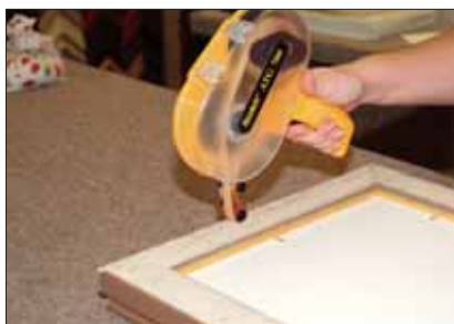
Photo 1: Applying the ATG tape in preparation for the backing paper.
