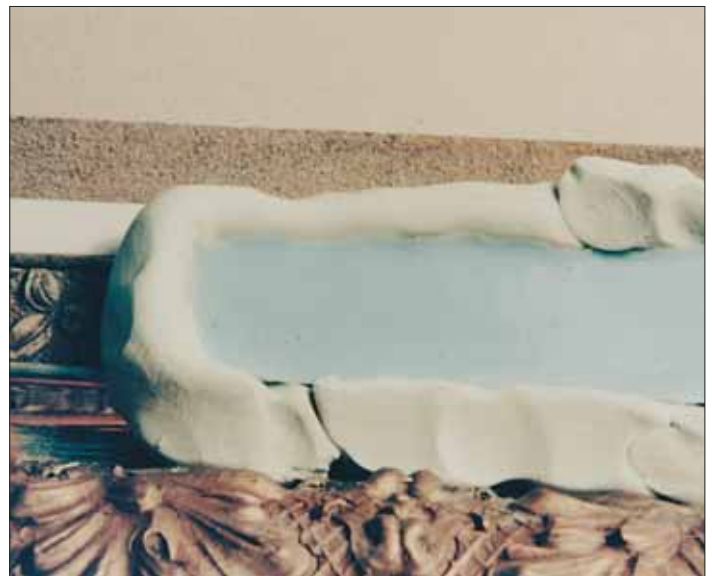
Photo 2: A clay dam is all that is needed to pour a mold of this antique frame.
