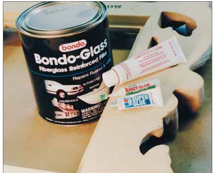
Photo 1: Shown here is a polyester resin filler and glues resting on the back of a polyurethane frame.
