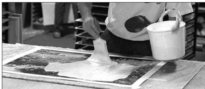
Photo 1: In order to "seize" the image, it can be laminated. However, many studios apply a liquid acrylic polymer as seen here.
