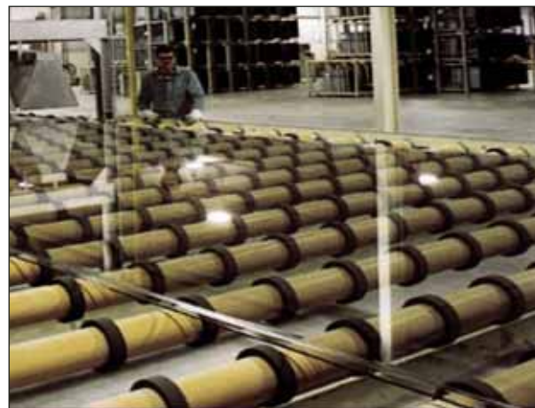
A continuous sheet of glass begins its exit from the manufacturing area, at the “cold end” of the float line.
