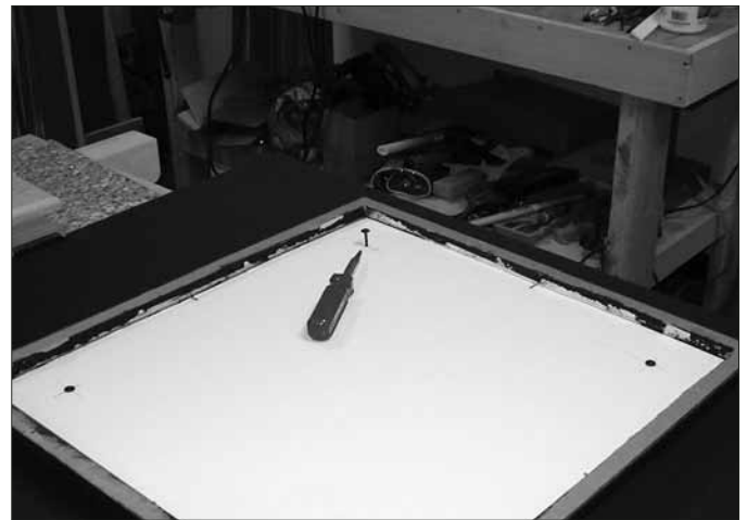
Photo 1. Round washer head screws can be used to center or position one object in relation to another without being exact when drilling.
