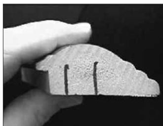
Photo 2: Nails should be inserted in the center two-thirds of the moulding, if the profile shape allows.
