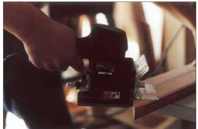
Photo 2: Operating the detail joiner. This joiner works similarly to the full-size joiner, which is the one used for wider mouldings.
