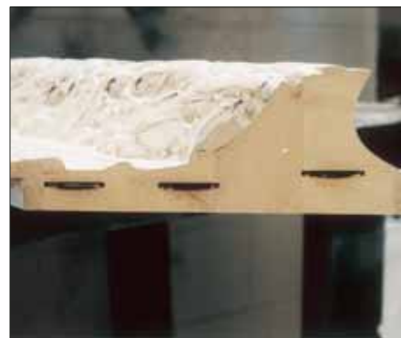
Photo 5: Miter edge showing biscuits in their grooves (Biscuits were colored black for better definition in this photo.)
