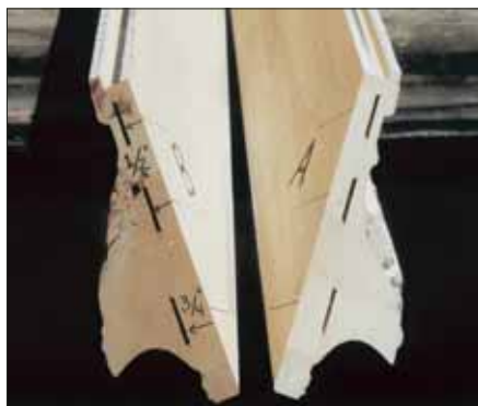
Photo 4: Ends of miter cuts showing the biscuit grooves, their depths, and placements
