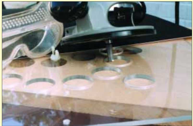
Holes were cut in the acrylic with a saw.
