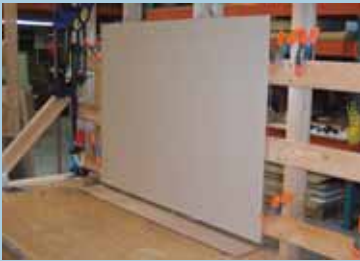
Photo C: The paper mask on the acrylic is peeled back 1" and the gluing process begins.
