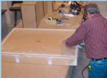
Photo F: The edges of the acrylic box is then sanded with an Orbital air sander.
