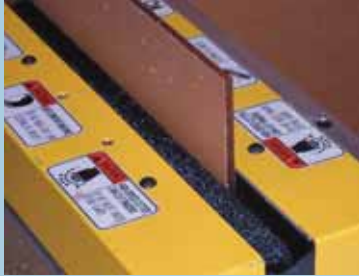
Photo B: Each piece is run through an edge finisher. This prepares for gluing.
