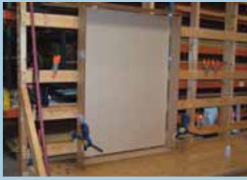
Photo D: The face and sides of the acrylic box have been glued and are clamped.
