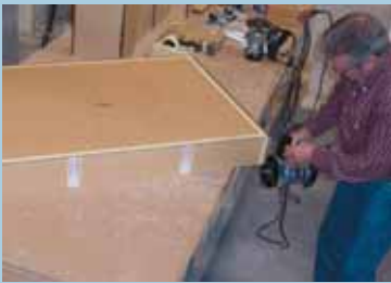
Photo E: The edges are taped next to the glued seams. Then routed with a bevel router bit.
