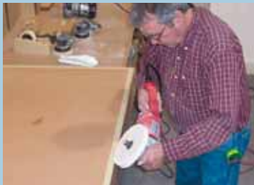
Photo H: The box is then buffed and polished on all the seams.
