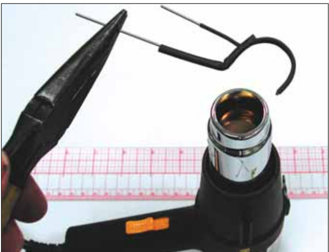
Photo 12: The shrink tubing conforms snugly to the shape of the mount when heat is applied. Shrink tubing is available from electrical/electronic parts distributors, in a number of colors and diameters. Radio Shack stores also carry a small assortment package.
