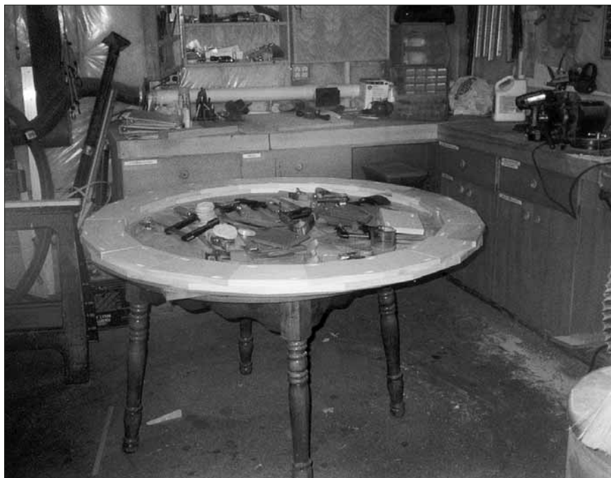
Photo 2: After the two 20-sided frames were built, they were glued to each other to form a roughly sized frame.
