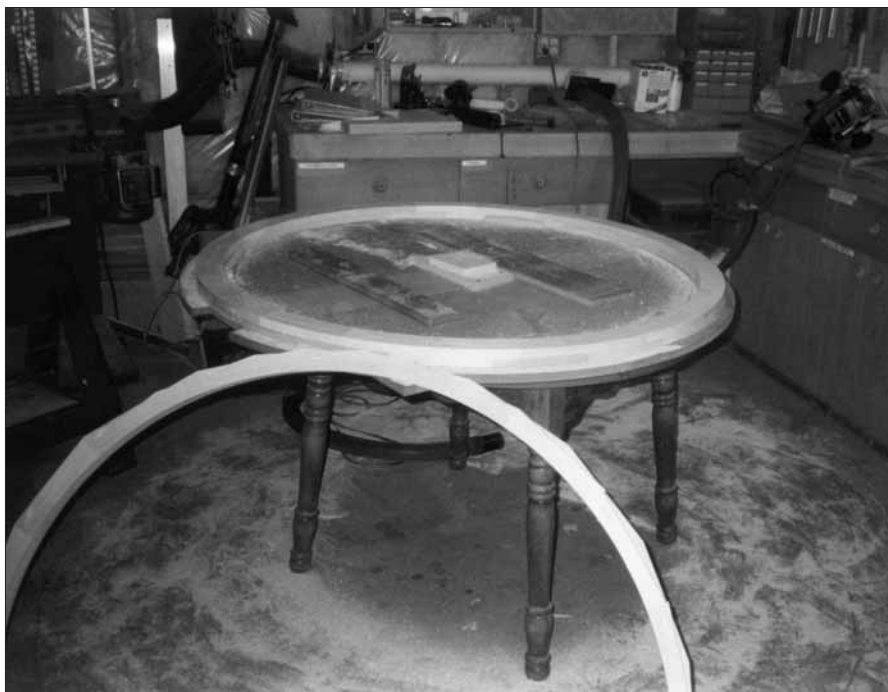
Photo 3: The frame shape to be used for the project (in the foreground) was routed from the 20-sided construction.
