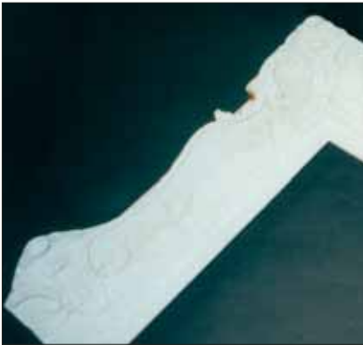
Photo 2: Apply Eaton ornamentation and hand carve sweep lines.
