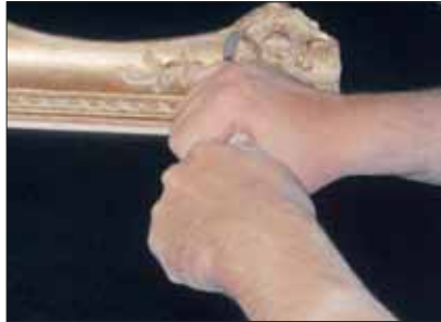
Photo 14: Burnishing the top edges. The frame is burnished and placed in the drying area for 20 to 35 minutes, depending on the humidity.
