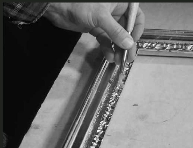
Photo 2: You can burnish with a small hook (or dog's tooth) agate to work on carving details.
