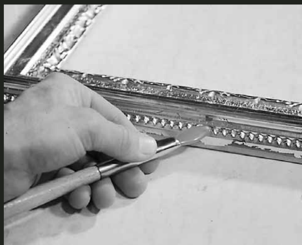
Photo 4: A spoon-shaped agate can be used to burnish the bead on the side of the frame. This agate shape combines both a flat and a curved shape. For that reason, it is ideal to use for burnishing almost any surface.
