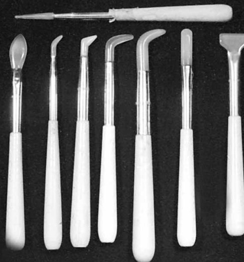
Photo 1: Agate burnishers come in a number of shapes and sizes. Shown here (left to right) are a spoon; then four of the hook (or dog's tooth) types; next, a straight with a rounded nose; and a flat. The burnisher along the top is a pointer. The burnisher you use depends on the shape of the frame profile you are burnishing, as well as your personal preference.
