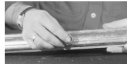
The frame is rubbed back to expose the bole with 0000 steel wool.
