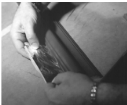
The leaf is rolled onto the surface of the moulding. This technique will eliminate most breaks in the frame.
