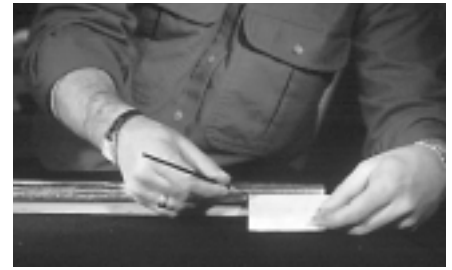
Lay lines imitate the look of real gold. They are placed with shellac, a small brush, and a 3" card.
