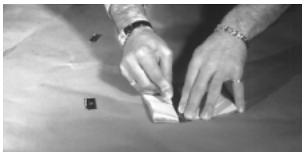
This book of leaf is pre-cut with a razor blade and straight-edge on a hard surface.
