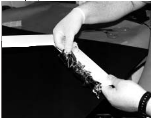
Once the metal leaf has been cut in thirds, it can easily be applied to the ATG.
