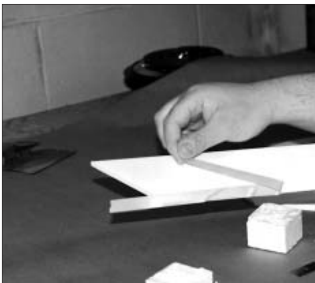
Metal leaf can be adhered to the bevel board with ATG tape. The entire bevel must be covered with ATG.
