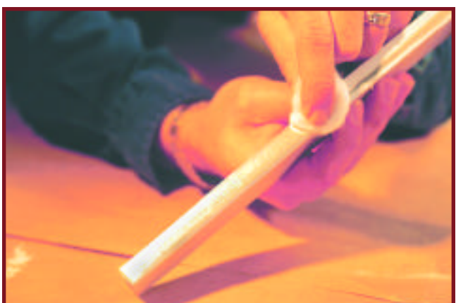
Wipe off the whiting and lacquer thinner paste with a cotton ball.
