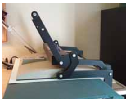
Photo 9: Readjust for Foam—Verify handle adjustment prior to laminating when using 1/2" overlay foam. Sometimes contracted 1/4" foam will not require the press to be readjusted, but 1/2" will always need to be.
