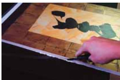
Photo 8: Trim Excess Laminate—Trim excess laminate from the edges of the sized mounted substrate to prevent laminate from bonding to anything else in the press, like the sides of the substrate or the sponge pad.
