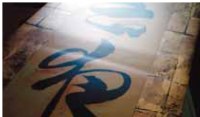
Photo 11: Dented Substrate—This substrate was dented during lamination even with a release board and overlay foam. This damage cannot be undone and the project will need to be replaced.
