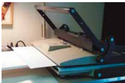
Photo 5: Pressure Adjustments—Check your mechanical press for proper pressure adjustments by placing the substrate and release board into the closed, but not locked, press. The arm should be 45° to the table with all layers inside.
