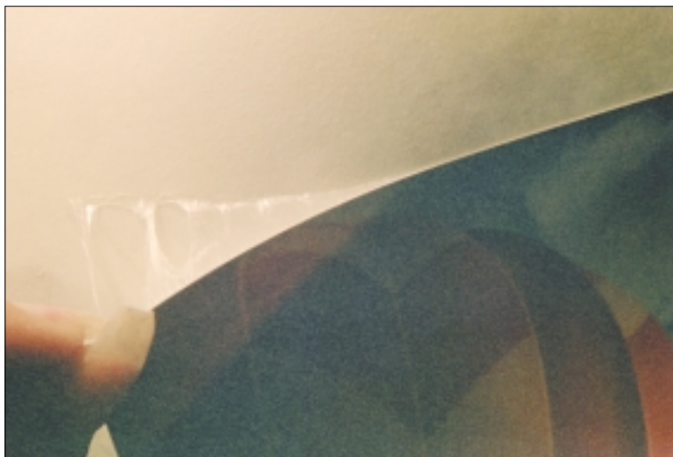
Photo 1: PMA (3M) Mounting film adhesive has only one release liner and no carrier, making this P-S film perfect for self-shaping. Two layers of film may be applied when bonding rough textures to make certain of full adhesive coverage.
