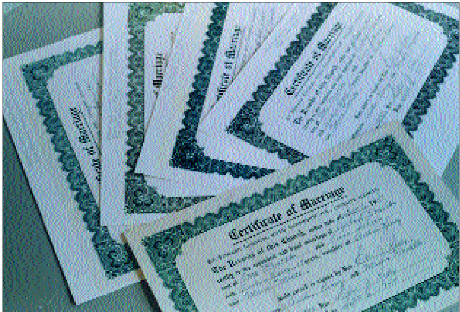
Photo 4: The photo shows the color variations between copiers. Lower right front is the aged, yellowed original; (l to r) Xerox 5765 added blue; Ricoh 5006 ghosted all lines with distortions; Canon 350 created a black outlined all colors; and Kodak Coloredge 1525, yes the green border corrected to black.
