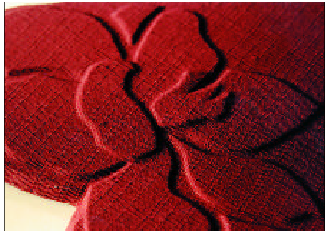
Photo 8: Double three-dimensional embossing requires two templates when mounting.
