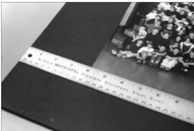
Photo 5: A 4" allowance is calculated into the board sizing for later bevel trimming.
