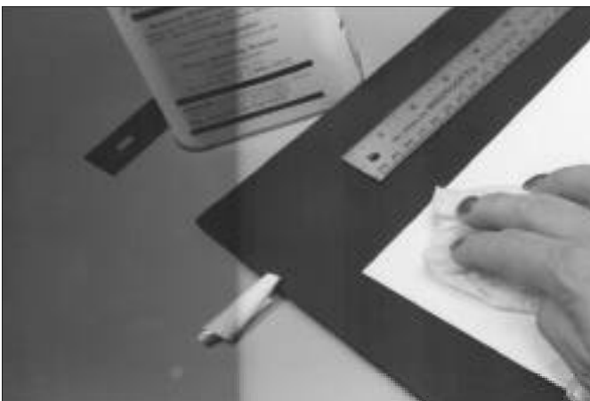
Photo 4: The peeled stickers left an adhesive residue which was easily removed with a standard solvent.
