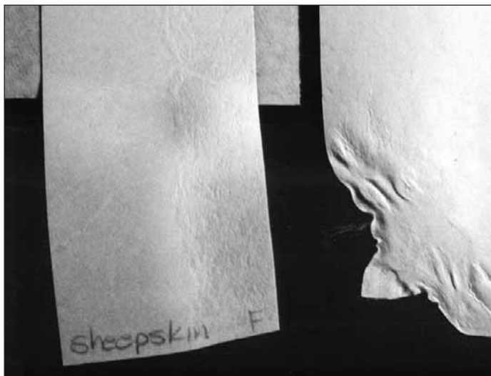
Photo 1: Sheepskin Samples—The left sample shows a scrap of sheepskin that has been dampened and air-dried. There is a slight natural shrinkage due to the stretching, cleaning, and dehairing process. The right sample shows the unfortunate damage resulting from the combination of heat and moisture when applied to parchment.
