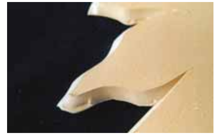
Photo 5: Using Old Blades—Same brand of foamboard demonstrated in Photo 4, but cutting was done with an old blade which snagged and pulled the inside.
