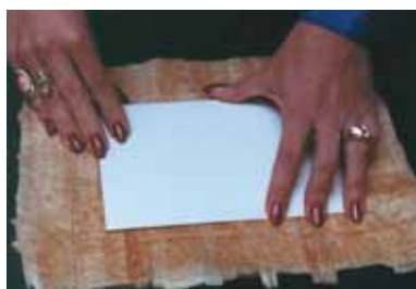
Photo 2: Seating the Fallout—By seating the fallout back into the window opening the papyrus will be forced into the shape of the opening, ensuring all the deep 3/16" foam bevels will be covered once wrapped.
