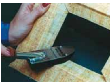
Photo 4: Reinforcing the Bevel—Since foamboard is a heat insulator, iron the bevel edge, making sure the flat of the iron is in total contact to the flat of the bevel in order to reactivate the adhesive and bond the papyrus to the bevel. Work well into the corners with the edge of the iron.
