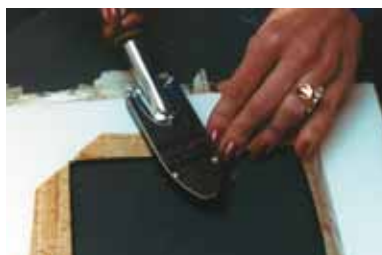
Photo 5: Ironing the Tabs—Once the bevels and corners are perfect, turn the mat face-down and iron the adhesive-backed tabs to the verso side of the mat opening.
