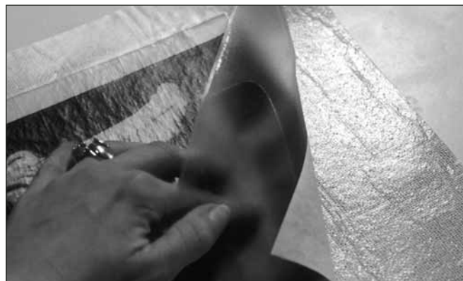
Photo 9: Heat-Activated (HA) Canvas Without Liner—If canvas has a dry adhesive with no protective liner, simply square up the sides of the decal with the liner.
