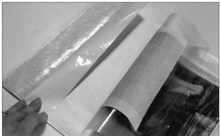
Photo 7: Heat-Activated (HA) Canvas With Liner—Fold back the removable liner a few inches to expose sticky adhesive. Square up decal from the protected bottom edge and align up sides to the top.
