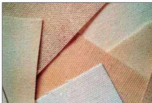
Photo 1: Canvas Textures, Weights, and Colors— There are numerous raw canvas textures available from coarse to fine weave, knobby uneven threads to even refined threads all determined by the thickness and tightness of the thread patterns in the fabric. Being comprised of assorted fibers, their colors vary.
