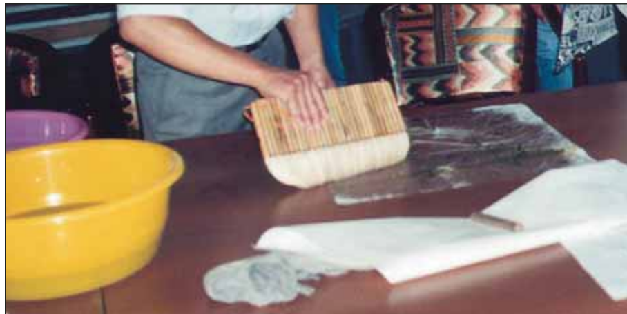
Photo 1: The honshi is laid face down and moistened with a wide soft hake brush.
