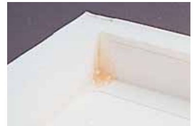
Photo 5: On large pieces (11"x14" and up), glue the sides in place then reinforce the adhesive by running a bead of hot glue all along the inner corner seam. Note tape on the right and glue on the left seams.
