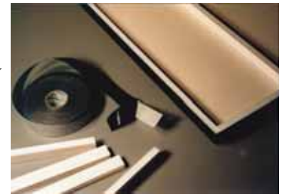
Photo 4: View of Back—This sample is mounted to 3/16" foam with 1/2" sides and 1 1/4" wide black linen tape.
