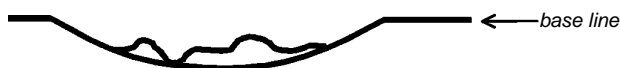
Diagram 1: The image area is often recessed into a concave shape with the embossed image projecting forward, but still behind the base line.
