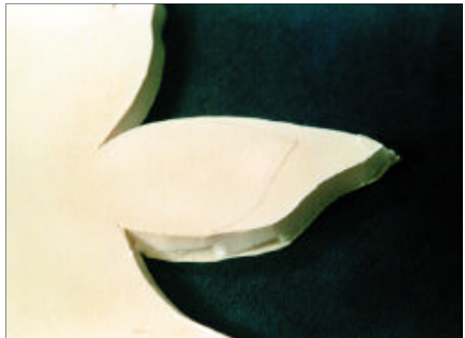
4B: Notice the extremely clean cut bevel with no irregularities in the foam.
