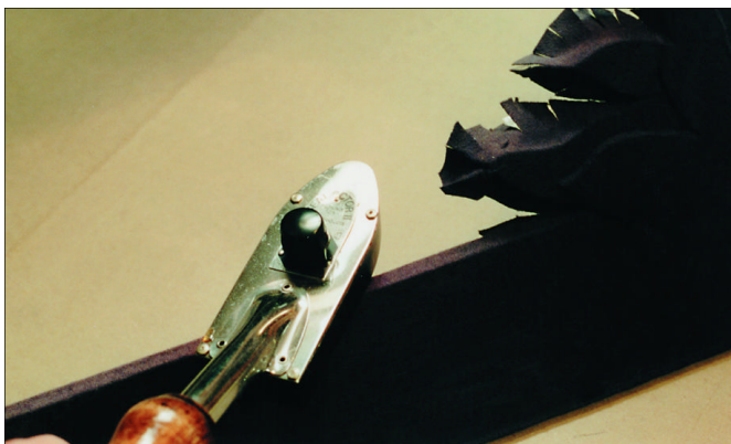
Photo 6: Iron the bevel to reactivate unmelted adhesive.
