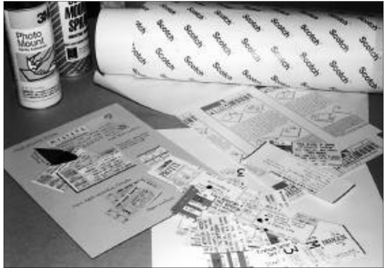
Any process of mounting that does not use heat is considered cold mounting. Wet, spray and pressure-sensitive boards and films all fit into this category whether a cold vacuum system is used with them or not.
