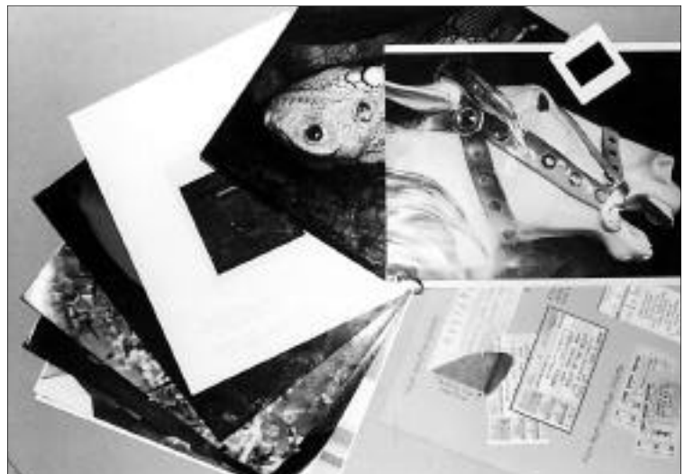
Clockwise from lower left: black and white RC photos (2), color RC (3), Polaroid print (1), Ilfochrome Classic (lizard), four-color photocopy (horse), tickets. All have same basic heat-sensitivity whether as produced orange-peel, thermo-graphic inks or paper.
