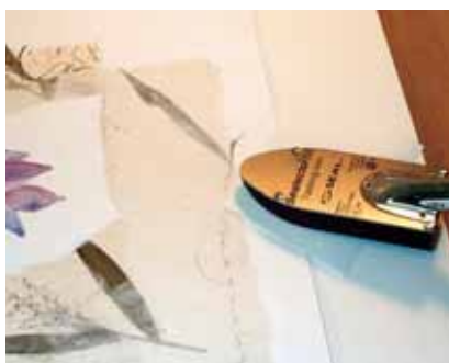
Photo 3: Tack—Since this mat unit was to be linen hinged along the left edge to the backing after mounting, tack the artwork in place after it has been centered beneath the mat prior to mounting.
