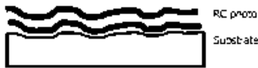
Diagram 1: Here is an illustration of orange peel. This occurs when heat and pressure relax an RC photo into the highs and lows of the substrate.
