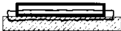
Diagram 2: An RC photo will never absorb adhesive for long-term bonding, but a fiber-based photo will. An adhesive must saturate both the item to be mounted and the substrate.
