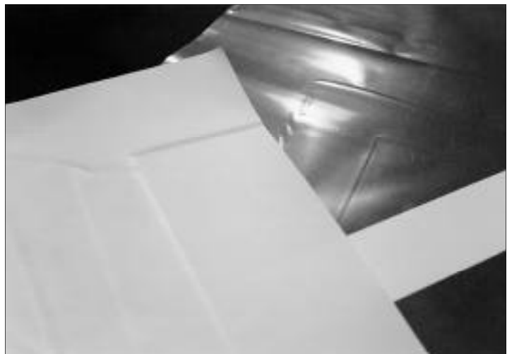
Samples of indented release papers and coated mylar. Remember to check your release materials periodically.
