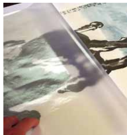
Photo 10: Re-aligning to Remove Air—With the tips of a gloved hand, a bone burnisher, or your clean fingernails roll the laminate back into place and the large bubbles will generally have been taken care of.
