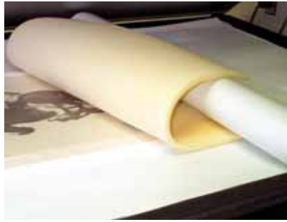
Photo 12: In the Press—The mounting package bottom to top consists of release paper, substrate, dry mount tissue, horse print, laminate, sponge overlay, topped with another sheet of release paper
