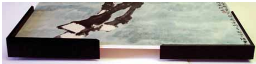
Photo 2: Moulding Options—The Matte Black anodized Nielsen Profile 34-21 (left) is 1\frac{3}{8} " deep with a \frac{7}{32} " surface lip that is \frac{3}{8} " down to the print. The Nielsen Profile 3-50 (right) is 1" deep with a small narrow \frac{3}{16} " lip that lays flat against the laminated print.
