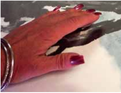
Photo 11: Checking for Air Bubbles—Check again for trapped air by running your fingertips gently across the laminate surface.
