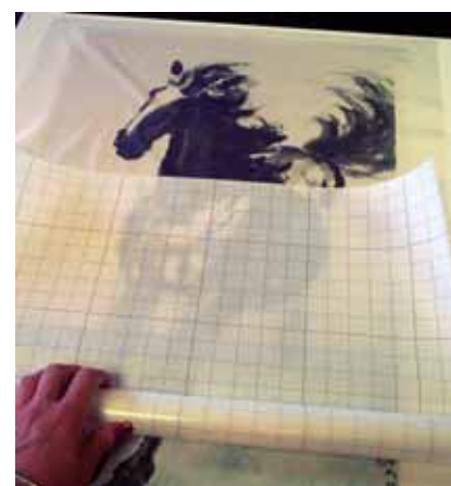
Photo 9: Rolling Off the Liner—Standing at the end of the project, allow the substrate to bump against you as you gently pull the remaining liner from the laminate, rolling it as it is pulled toward you.
