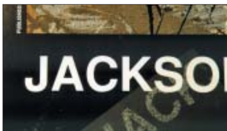
Photo 3: Some of the surface ink remained as ghosted white ink on the adhesive side of the laminate when peeled up for repositioning after 15 minutes of contact.
