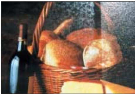
Photo 4: Forgotten Foam —The central top area of this image shows the scuffed laminate which is the result of forgetting overlay foam in the laminating package. The far right section is correctly laminated with foam.
